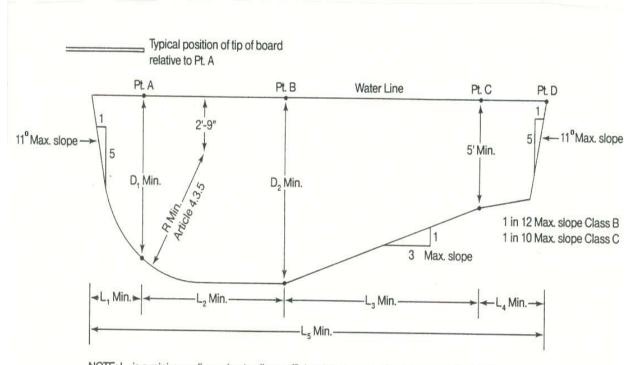
NOTE:  $L_4$  is a minimum dimension to allow sufficient length opposite the board. This may of course be lengthened to form the shallow portion of the pool.
